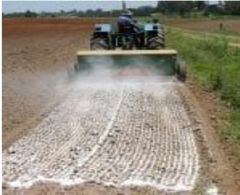
Figure 4: The grass seed or wheat seed planter lime applicator.
