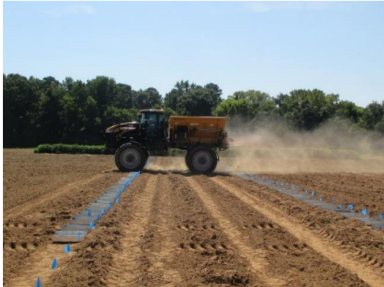
Figure 1: containers spaced to determine the amount of agricultural lime applied.
