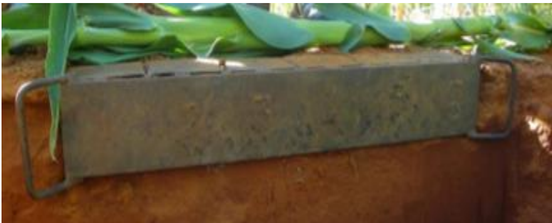
Figure 2: Steel plate to take soil samples. (Photo supplied by Jan du Toit Agricultural adviser: Omnia).
