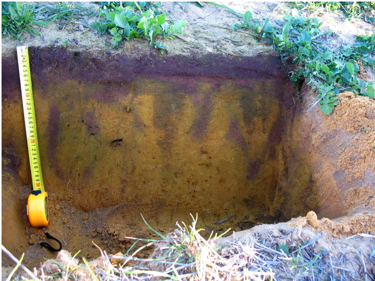
Figure 6: Effectivity of deep incorporation of lime. (Photo provided by Chris Gazey 2014). The purple colour indicates a high pH and lime that has not fully reacted with the soil and zones where lime has been incorporated deeply after application on the surface.
