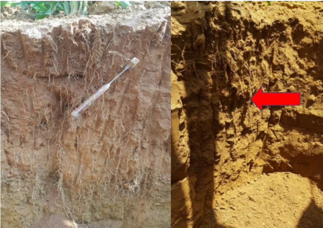
Figure 1: Soil profile inspection to determine root development (Photo supplied by Kobus van Zyl, 2020).
